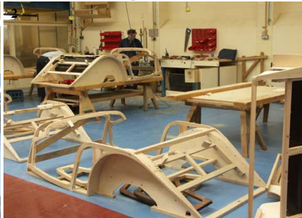
2 We were then free to wander through the workshops watching the craftsmen assemble the skeletons of the cars. Jobs at the Morgan factory are much sought after with over 140 applicants for just one position
