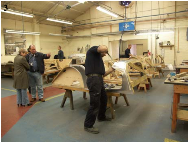
3 Here we watched how the aluminium is laid over the wooden frame, buffed and polished in preparation for the paintshop.
